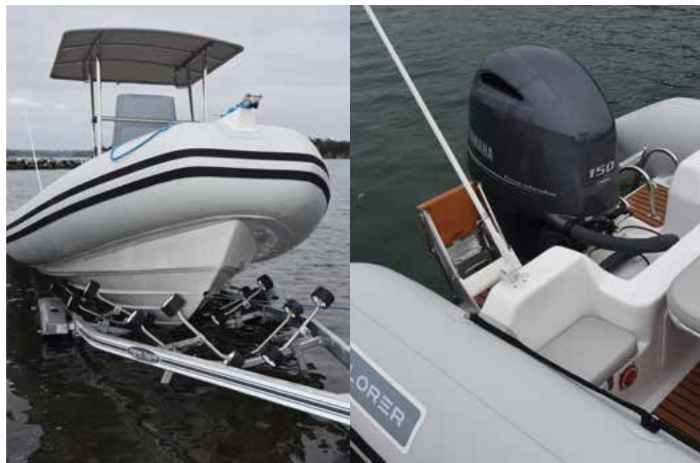
The raised bow along with the large diameter tubes set on broad flanges make this a very dry boat.
