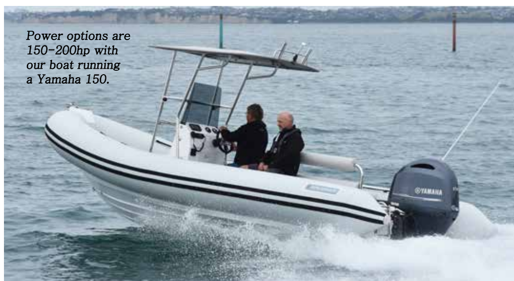
The raised bow along with the large diameter tubes set on broad flanges make this a very dry boat.
