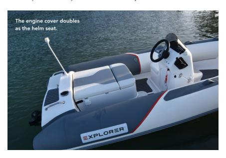
Boat Design Name Viking 420 Jet RIB Year Launched: 2020 / New Zealand Builder Explorer Boats Price as Tested \$NZ47,000 LOA 4.20m Beam 1.98m Deadrise 5 deg Construction Fibreglass hull / Hypalon Orca Tubes Weight: (boat only) 365 kg Trailerable Wgt 550 kg Power Type: amaha TR1 / Jet Max Horsepower 125 hp Max Speed 30 knots Fuel Capacity 50 litre Flooring U-Deck Trailer Hoskings Boat Supplied by Explorer Boats, Ph +64 9 412 2040 | andy@explorerboats.co.nz | www.explorerboats.co.nz
